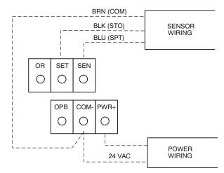
NOTE: Must use a separate isolated transformer.
